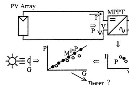
Figure 9: Analysing monitoring data
