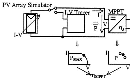
**Figure 3:** Static laboratory measurements
