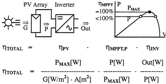
**Figure 2:** Efficiencies of MPPT and Power Conversion
