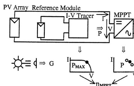
Figure 6: Using a calibrated reference module
