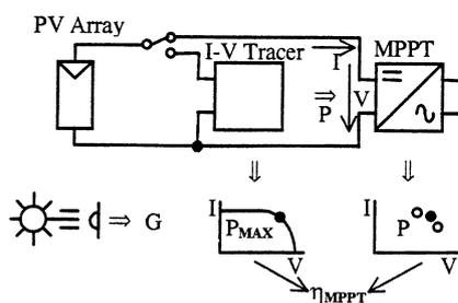
Figure 5: Switching between inverter and IV tracer
