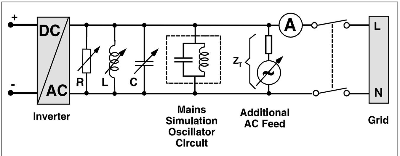
**Fig. 8:** Circuit to test the automatic isolation under islanding conditions according to new German regulation. The mains simulation oscillator circuit consists of a L and a C consuming  $Q = \pm 100 \text{ Var}$  . Additional AC feed: 30% of inverter power.
