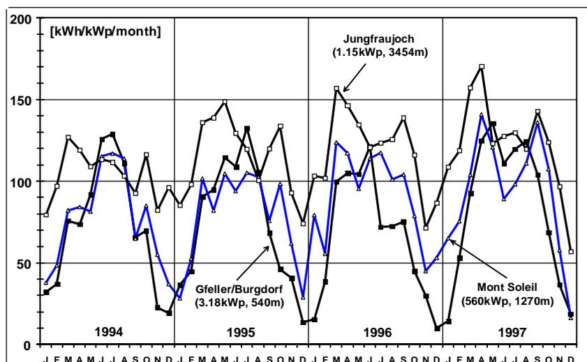
**Fig. 7:** Normalized monthly energy production (referred to nominal PV generator power) of PV plants Jungfrauoch (1.152kWp), Mont Soleil (560kWp) and Gfeller/Burgdorf (3.18kWp) in the years 1994 to 1997.
