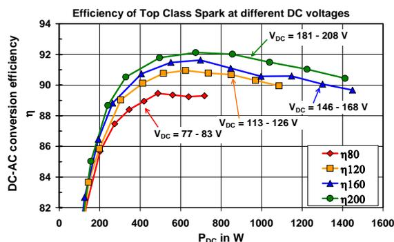
Fig. 4: DC-AC conversion efficiency of a Top Class Spark at different DC input voltages.
