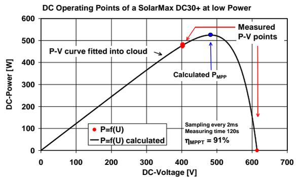
Fig. 9: Cloud diagram of a SolarMax DC30+ (30 kW) and P-V-curve fitted into diagram using least squares fitting through cloud and  $V_{OC}$  to determine  $P_{MPP}$ . At low power levels, the device operates at the minimum operating voltage of 400V. Therefore, if  $V_{MPP}$  is higher,  $\eta_{MPPT}$  must be lower, here only 91%. Loss of exact MPP-tracking at low power levels is typical for most inverters.
