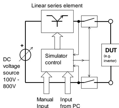
**Fig. 1: Block diagram of the PV generator simulators developed at HTI's PV laboratory.**
