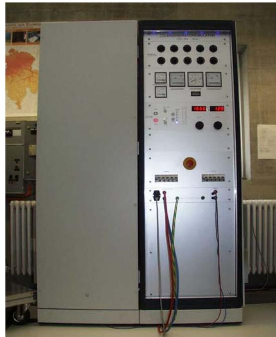
**Fig. 2: View of the PV generator simulator with  $V_{OC} \leq 750V$ ,  $I_{SC} \leq 40A$ ,  $P_{MPP} \leq 25kW$ .**
