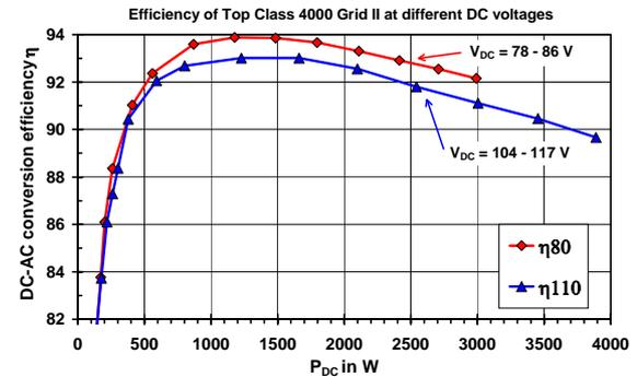
Fig. 5: DC-AC conversion efficiency of a Top Class 4000 Grid II at different DC input voltages.
