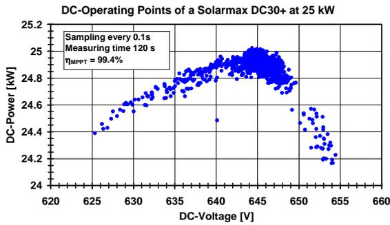
Fig. 6: Cloud diagram of an inverter Solarmax DC30+ operating at the I-V-curve of the PV simulator of fig. 3. Measured  $\eta_{MPPT}$  was 99.4%, MPP-tracking is very good.
