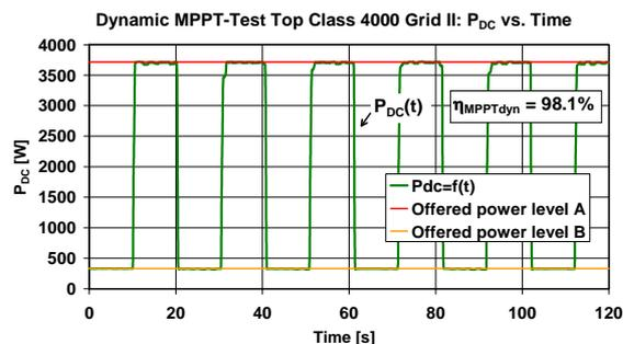
Fig. 11: Measured absorbed DC power  $P_{DC}(t)$  of an inverter with a very good dynamic MPP-tracking. Measured  $\eta_{MPP\text{TDyn}}$  is 98.1% according to (3), thus very high.
