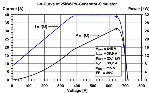
Fig. 3: I-V-curve (with fold-back current-limitation) of the highly stable 25kW PV-generator-simulator developed by HTI's PV laboratory.
