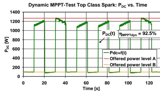
Fig. 12: Measured absorbed DC power  $P_{DC}(t)$  of an inverter with an average dynamic MPP-Tracking behaviour. Measured  $\eta_{MPP\text{TDyn}}$  is 92.5% according to (3).
