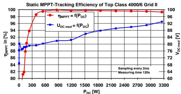
Fig. 10: Measured  $\eta_{MPPT} = f(P_{DC})$  for a TOP Class 4000 Grid II operating on an I-V-curve with relatively low  $V_{OC}$ . Power is varied indirectly by varying the current  $I$  on a given I-V-characteristic of the PV array simulator. Besides  $\eta_{MPPT}$  also the average DC operating voltage  $V_{DC}$  is indicated in the same diagram. For DC-voltages lower than 80 V the inverter gets problems with MPP-tracking and therefore  $\eta_{MPPT}$  is lower there.
