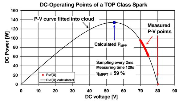
Fig. 8: Cloud diagram of a Top Class Spark (1.3 kW) and P-V-curve fitted into diagram using least squares fitting through cloud and  $V_{OC}$  to determine  $P_{MPP}$ . As  $V_{OC}$  of the simulated array is too low here,  $V_{MPP}$  is lower than the lower limit of the tracking window, therefore the MPP can not be found and measured  $\eta_{MPPT}$  is only 59 %.
