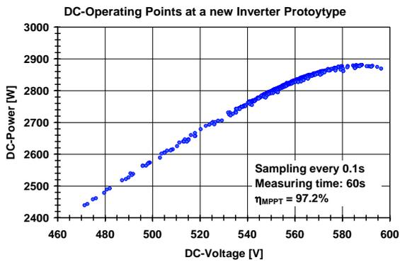
Fig. 7: Cloud diagram of a prototype of a new inverter. Measured  $\eta_{MPPT}$  was 97.2%, it is obvious that this device has a sporadic MPPT-problem.
