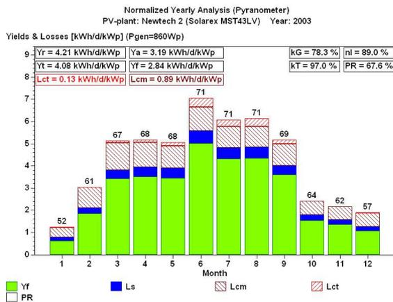
**Fig. 5: Normalised yearly analysis for 2003 of PV plant Newtech 2 with a-Si modules MST43-LV. Specific annual Energy yield 2003: 1037 kWh/kWp, PR = 67.6%, winter energy fraction 28.6%. Due to degradation, PR is considerably lower than in 2002.**
