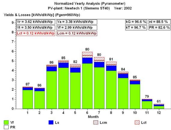
**Fig. 2: Normalised yearly analysis for 2002 of PV plant Newtech 1 with CIS-modules Siemens ST40. Specific annual energy yield 2002: 1091 kWh/kWp, PR = 82.6%, winter energy fraction 31.8%.**
