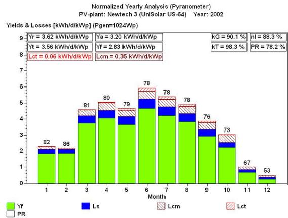
**Fig. 6: Normalised yearly analysis for 2002 of PV plant Newtech 3 with a-Si modules Unisolar US-64. Specific annual Energy yield 2002: 1033 kWh/kWp, PR = 78.2%, winter energy fraction 31.1%. Starting in October, PR decreases considerably due to module degradation.**
