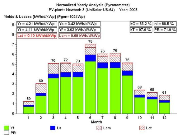
**Fig. 7: Normalised yearly analysis for 2003 of PV plant Newtech 3 with a-Si modules Unisolar US-64. Specific annual Energy yield 2003: 1102 kWh/kWp, PR = 71.9%, winter energy fraction 28.6%. Due to degradation, PR is considerably lower than in 2002.**
