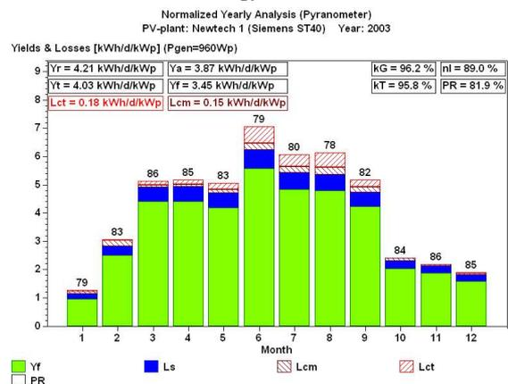
**Fig. 3: Normalised yearly analysis for 2003 of PV plant Newtech 1 with CIS-modules Siemens ST40. Specific annual energy yield 2003: 1259 kWh/kWp, PR = 81.9%, winter energy fraction 32.0%. A minor production loss could be observed only during the hot an dry summer months.**
