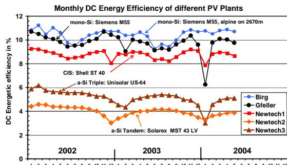
**Fig. 8: Monthly DC energy conversion efficiency of the three PV plants Newtech 1 to 3 and of two PV plants with mono-c-Si (alpine plant on 2670m).**
