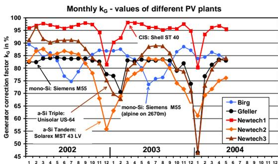
**Fig. 9: Monthly values of the generator correction factor  $k_G = Y_a/Y_T$  of the three Newtech plants and of 2 plants with mono-c-Si cells (alpine plant on 2670m).**
