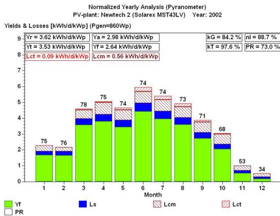
**Fig. 4: Normalised yearly analysis for 2002 of PV plant Newtech 2 with a-Si modules BP Solarex MST43-LV. Specific annual Energy yield 2002: 964 kWh/kWp, PR = 73.0%, winter energy fraction 30.4%. Starting in October, PR decreases considerably due to module degradation.**
