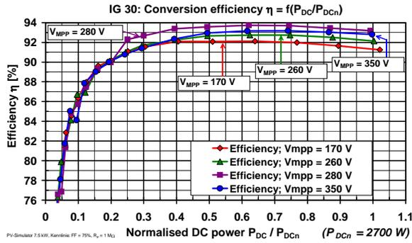
**Fig. 2:** Measured conversion efficiency of an inverter IG 30 with galvanic separation (thus a little lower  $\eta$ ) at four different DC-voltages ( $P_{DCn} \approx 2,7 \text{ kW}$ ).
