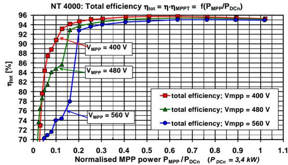
**Fig. 9:** Total efficiency  $\eta_{tot}$  of a NT4000 vs. normalised MPP-power  $P_{MPP}/P_{DCn}$  at 3 different MPP voltages. Because of the relatively low  $\eta_{MPPT}$  at low power levels and higher values of  $V_{MPP}$ , despite the high conversion efficiency  $\eta$  the device has a relatively low  $\eta_{tot}$  there.
