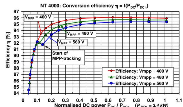
**Fig. 1:** Measured conversion efficiency of an inverter NT4000 without transformer at three different DC-voltages ( $P_{DCn} = 3,4kW$ ).
