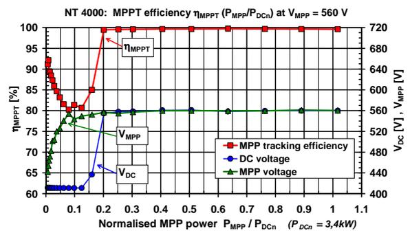
**Fig. 5:** MPP tracking efficiency  $\eta_{\text{MPPT}}$  of an inverter NT4000 vs. normalised MPP-power  $P_{\text{MPP}}/P_{\text{DCn}}$  at  $V_{\text{MPP}} \approx 560 \text{ V}$ . As the inverter operates at low power levels at the lower voltage  $V_{\text{DC}} \approx 410 \text{ V}$ ,  $\eta_{\text{MPPT}}$  is lower there. For higher power levels,  $\eta_{\text{MPPT}}$  rises towards 100%, as  $V_{\text{DC}} \approx V_{\text{MPP}}$ .
