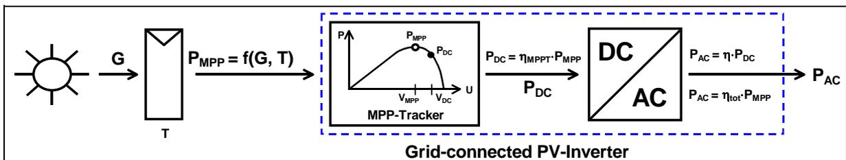
**Fig. 9:** Determination of total efficiency  $\eta_{tot}$  of grid-connected PV inverters:
