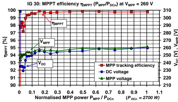
**Fig. 6:** MPP tracking efficiency  $\eta_{MPPT}$  of an inverter IG30 vs. normalised MPP-power  $P_{MPP}/P_{DCn}$  at  $V_{MPP} \approx 260$  V. Even at low power levels, the deviation of  $V_{DC}$  compared to  $V_{MPP}$  is low, therefore static MPP-tracking behaviour is very good also there.
