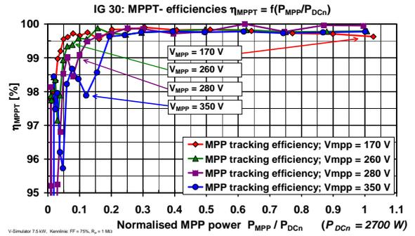
**Fig. 8:** Static MPP tracking efficiency  $\eta_{MPPT}$  of a IG30 vs. normalised MPP-power  $P_{MPP}/P_{DCn}$  at 4 different MPP voltages. Compared to fig. 7, the scale for  $\eta_{MPPT}$  is considerably extended. Static MPP tracking of this device is very good also at low power levels.
