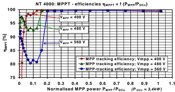
**Fig. 7** Static MPP tracking efficiency  $\eta_{MPPT}$  of a NT4000 vs. normalised MPP-power  $P_{MPP}/P_{DCn}$  at 3 different MPP voltages. As the device operates at a fixed voltage  $V_{DC} \approx 410$  V at low power,  $\eta_{MPPT}$  is lower than 100% there (depending on actual location of  $V_{MPP}$ ).
