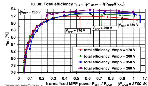
**Fig. 10:** Total efficiency  $\eta_{tot}$  of an IG30 vs. normalised MPP-power  $P_{MPP}/P_{DCn}$  at 4 different MPP voltages. At low power, owing to the good MPP-tracking, for  $\eta_{tot}$  the device can compensate most of the lower conversion efficiency.
