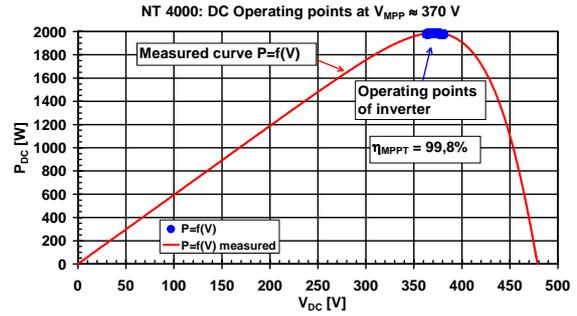
**Fig. 3:** Cloud diagram of an inverter NT4000 at  $P_{\text{MPP}} \approx 2 \text{ kW}$  and  $V_{\text{MPP}} \approx 370 \text{ V}$ . Measured  $\eta_{\text{MPPT}}$  is 99,8%, MPP-tracking is very good here.
