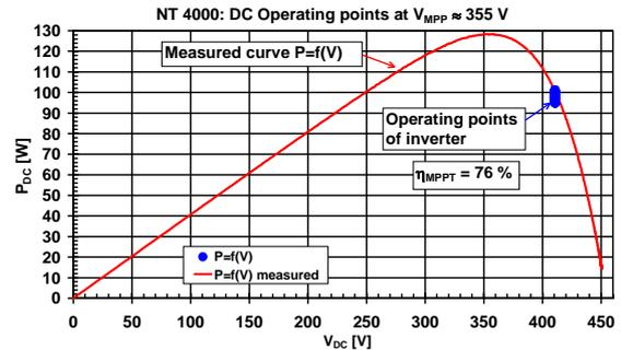
**Fig. 4:** Cloud diagram of an inverter NT4000 at  $P_{\text{MPP}} \approx 130 \text{ W}$  and  $V_{\text{MPP}} \approx 355 \text{ V}$ . The inverter operates at  $V_{\text{DC}} \approx 410 \text{ V}$  far away from the MPP. Measured  $\eta_{\text{MPPT}}$  is 76%, MPP-tracking is rather bad here.
