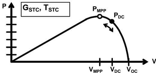
**Fig. 2:** P-V-curve of a PV array at standard test conditions (STC),  $G = G_{STC} = 1 \text{ kW/m}^2$ , cell temperature  $T_C = 25^\circ\text{C}$ .
