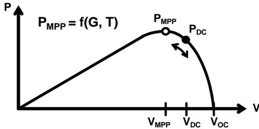
**Fig. 1:** The P-V-curve of a PV array depends on irradiance  $G$  into the array plane and on cell- or module temperature  $T_C$ . Thus also maximum power  $P_{MPP}$  of the PV array at the maximum power point (MPP) of the array depends on  $G$  and  $T_C$ .
