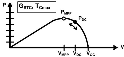
**Fig. 4:** P-V-curve of a PV array at  $G_{STC} = 1 \text{ kW/m}^2$  and maximum expected cell temperature  $T_{Cmax}$  (e.g.  $55^\circ\text{C}$  to  $65^\circ\text{C}$  for plants in moderate climates at lower locations).
