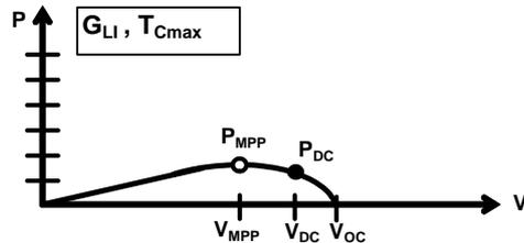
**Fig. 5:** P-V-curve of a PV array under hot, but cloudy weather conditions after a sudden drop of irradiance down to  $G_{LI} < G_{STC}$ .
