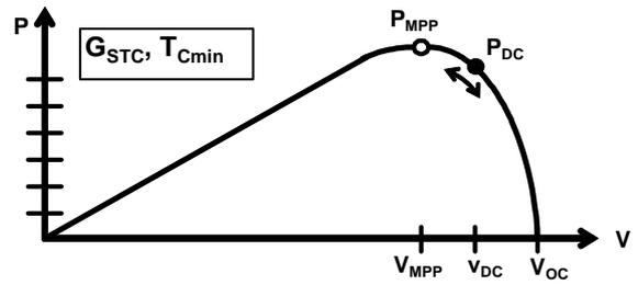
**Fig. 3:** P-V-curve of a PV array at  $G_{STC} = 1 \text{ kW/m}^2$  and minimum expected cell temperature  $T_{Cmin}$  (e.g.  $-10^\circ\text{C}$  for plants in moderate climates at lower locations).
