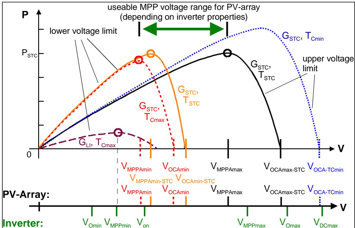
Fig. 7: Usable MPP-voltage range at  $G_{STC} = 1 \text{ kW/m}^2$  for a PV array (voltage values over the arrow) determined according to the indications on the inverter data sheet (below the arrow)
