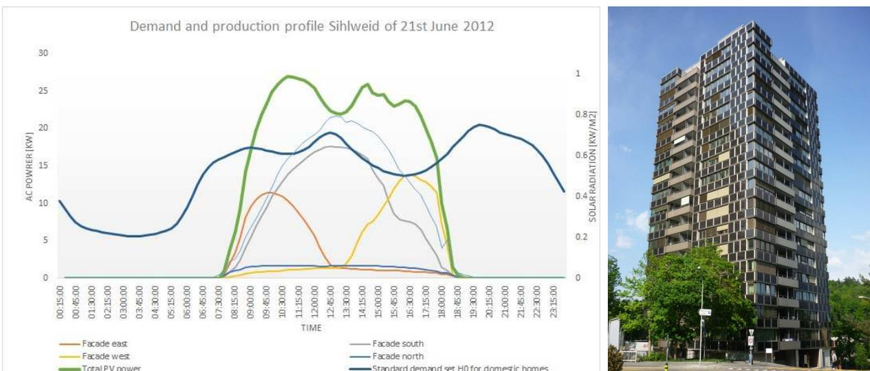
Fig. 1 + 2: PV façades generate more constant solar power and increase the coverage of energy load.
