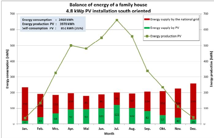
Fig. 3 + 4: Coverage of energy consumption through PV supply with different oriented PV installations. Conventional south oriented installation on a family house and apartment building with east-west oriented PV installation (inclination 45°).
