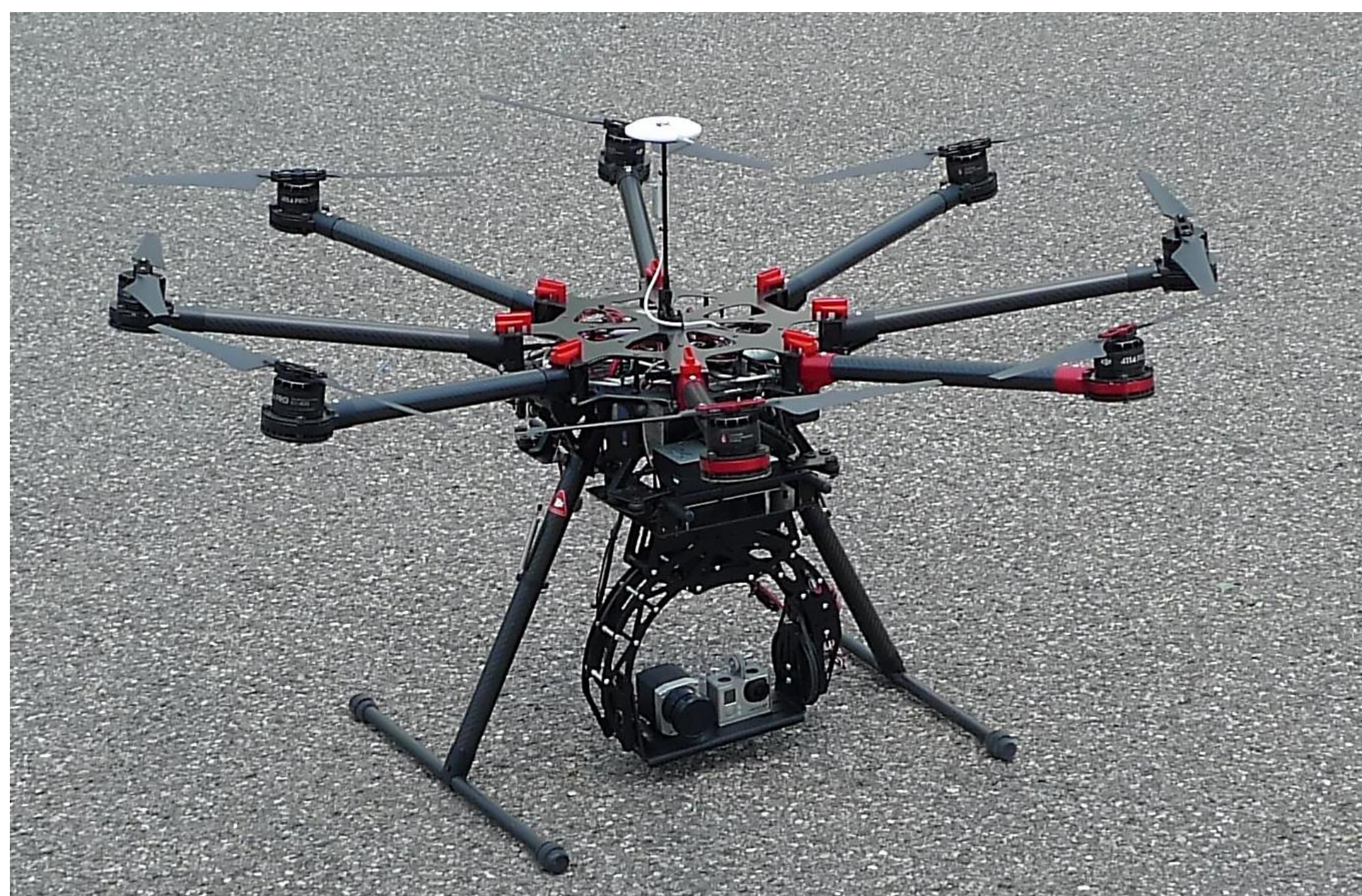
Fig. 1: PV LAB IR-multicopter drone; the take-off weight is about 7.5 kg.
